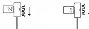
Fig.170 shows a gear tooth sensor where a ferrous metal concentrator is used. Use of a concentrator produces a greater field change and allows greater separation of the sensor and gear teeth.
